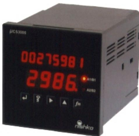
The CS 3000 series Flow Integrator Totalizers are precision instruments used along with flow meters, flow transmitters to indicate the instantaneous flow rate and carry out the totalization of flow. Two set-points are provided which can be configured on flow rate or on batches and hence can be used as batch controllers.
